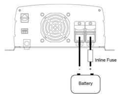
Figure 16. Battery cabling
