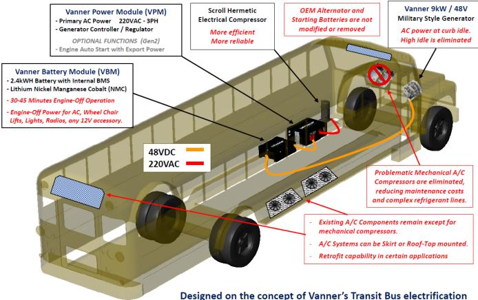
Designed on the concept of Vanner's Transit Bus electrification technology, currently operating on over 5000 buses worldwide.
